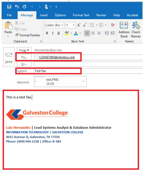
4. Confirm that the fax is filled out correctly and contains the documents you want to fax over as attachments. Click on the send button to send the fax to the recipient. After you click on send, XMedius will attempt to send the fax out via email. When the attempt is completed, an email confirmation will be sent to your inbox informing you that the fax was either successful or has failed. Below is an example of a successful fax being sent out via email:
